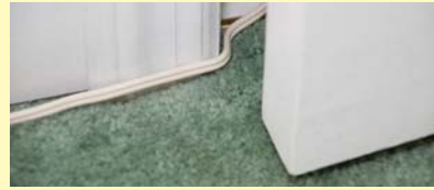
Damaged power supply cord (Example: door continually "pinches" cord)
