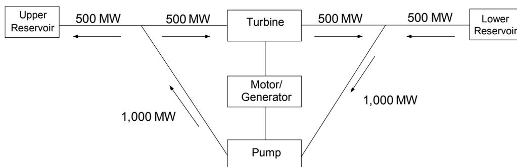
Figure 3 - A Ternary Power Hydro Unit Operating in the Hydraulic Short Circuit
