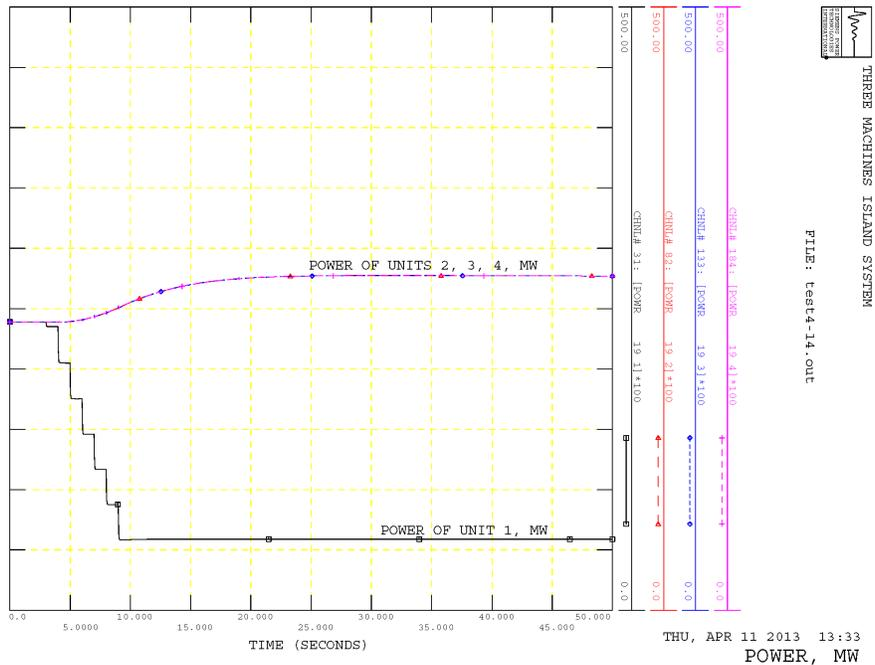
Figure 6 - Response of the Power of Units 2, 3, and 4 to a Step Reduction in the Power of Unit 1 with Four Units Sharing a Common Penstock
