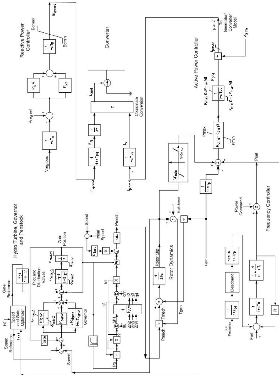
Figure 4 - Block Diagram of the AS PSH Turbine Model
