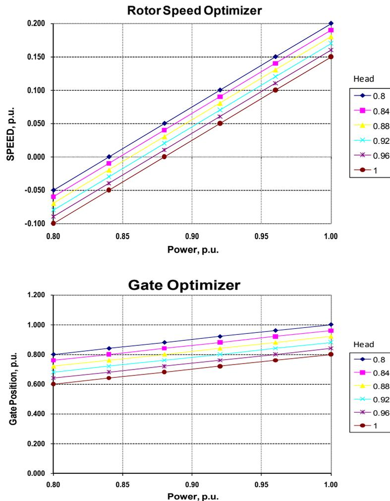
Figure 5 - Example of Speed and Gate Optimizer Characteristics Based on Analysis of Existing Projects
