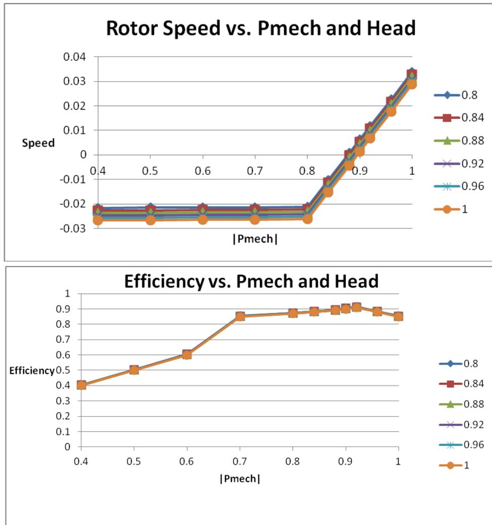
Figure 8 - Example of Speed and Gate Optimizer Characteristics for AS PSH Pump Based on Analysis of Existing Projects
