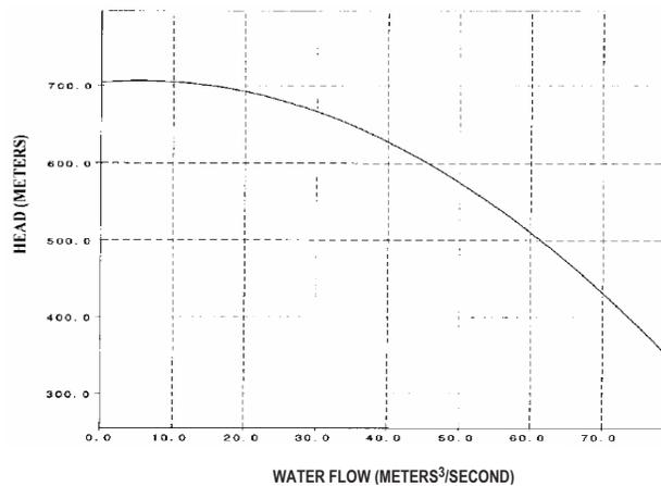
Figure 9 - Pump Head Characteristic
