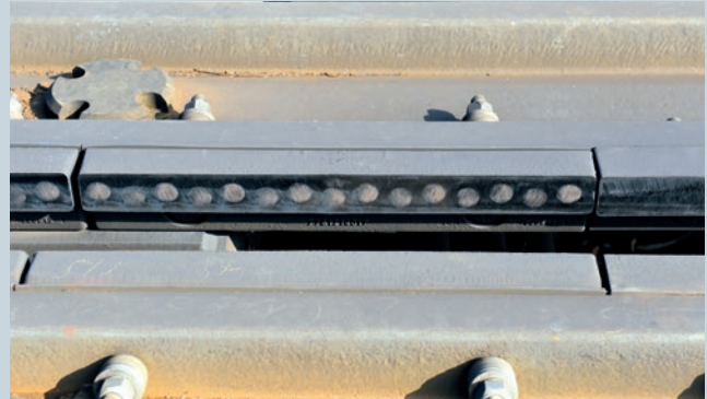
Retarder segment (braking beam with PUCK inserts)
